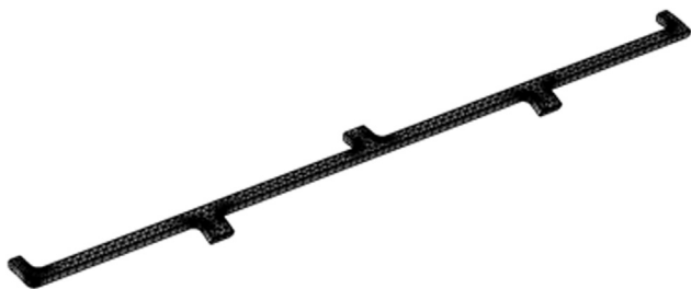
Figure 1 The meshed geometry of stent. Only 1/24 of the stent was simulated due to the symmetry of the model.
