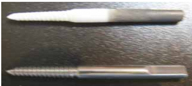
Figure 2 Half pins with and without hydroxyapatite and antibiotic coating.
