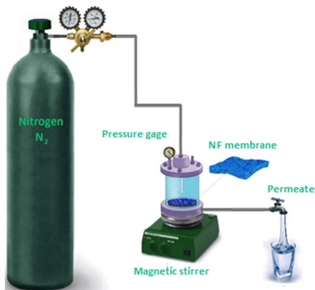
Fig. 1 Schematic flow diagram of the dead-end experimental cell
