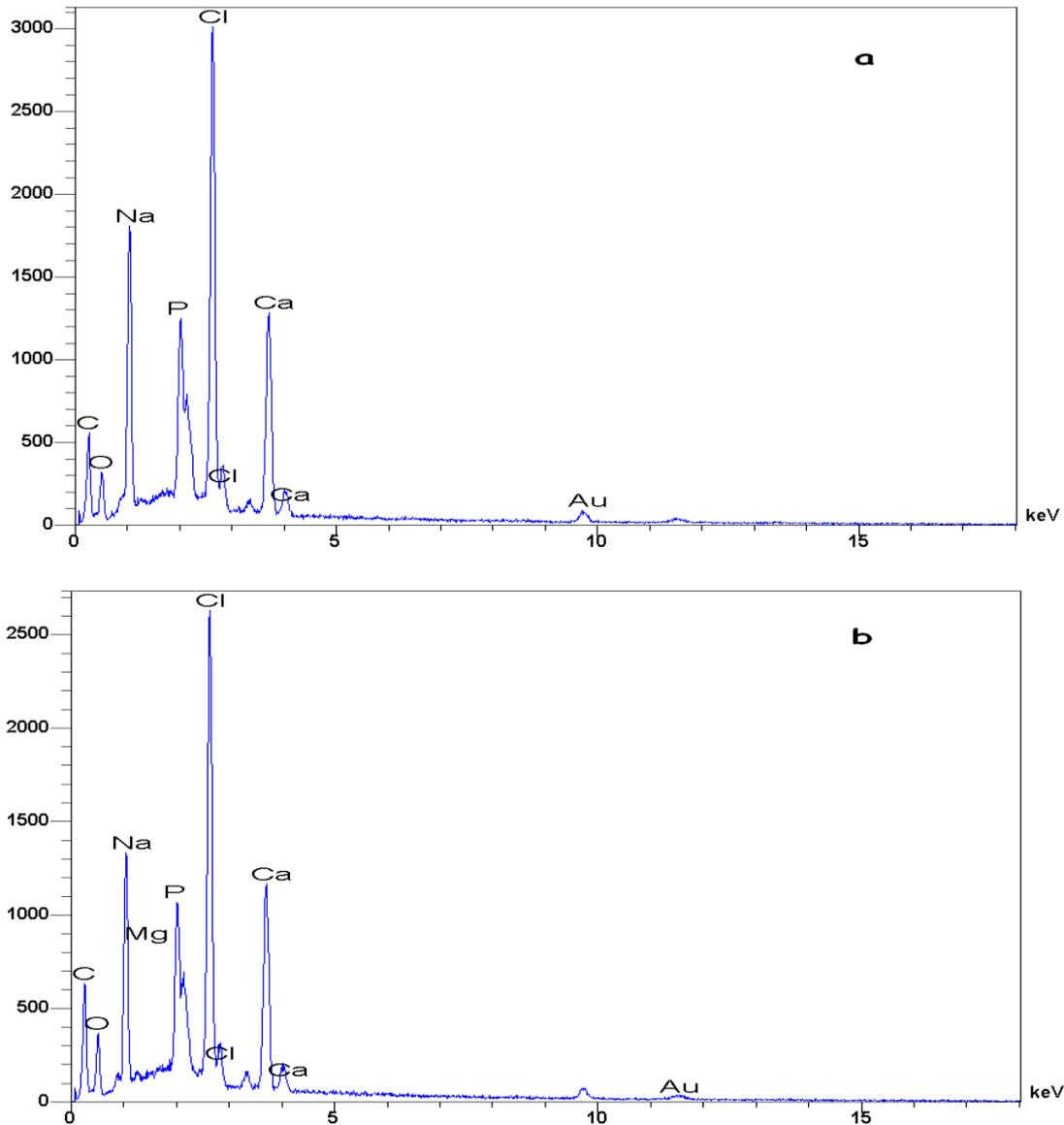
**Figure 8.** The EDS spectrum obtained from nanocomposite samples containing GEL and precipitated minerals formed related to samples of source of (a) Ca and (b) (Ca+20%Mg).
