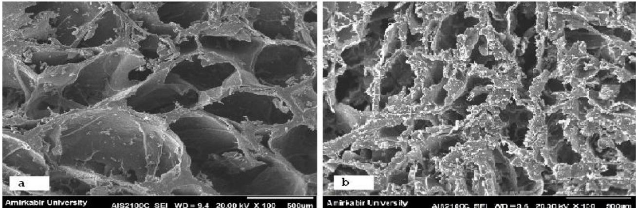
**Figure 7.** SEM micrographs obtained from surface of the synthesized biomimetic nanocomposite scaffold showing porous structure and nucleation and growth of the precipitate-phase nanocrystals on the surface of pore walls after being soaked in SBF solution (a) for source of Ca (b) source of (Ca+20%Mg)
