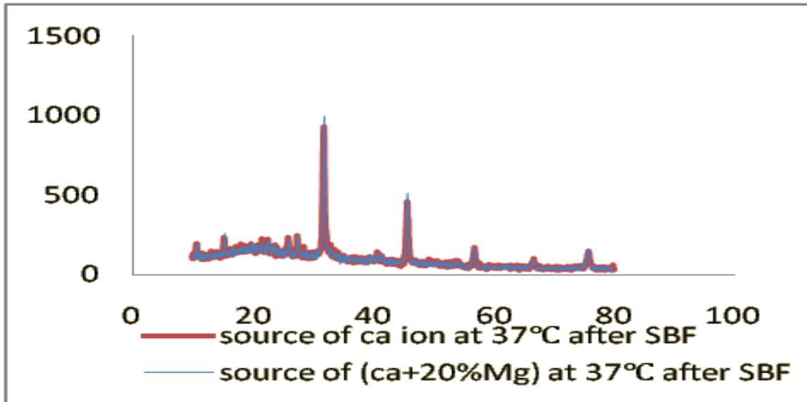
**Figure 4.** XRD spectra for source of Ca at 4°C and (Ca+20%Mg) at 37°C.
