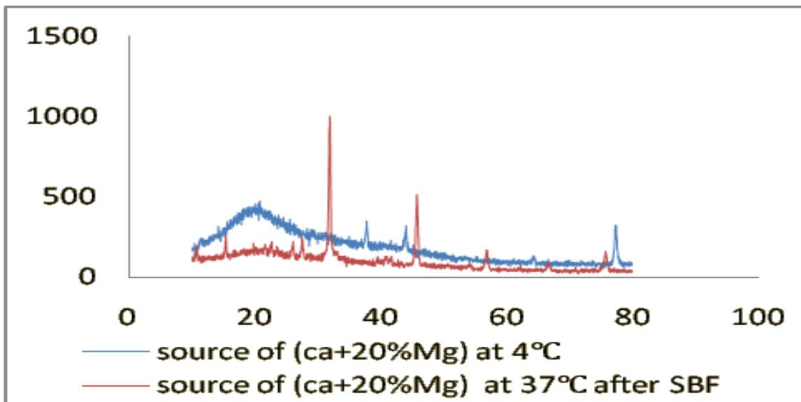
**Figure 6.** XRD spectra for source of (Ca+20%Mg) at 4°C and 37°C.
