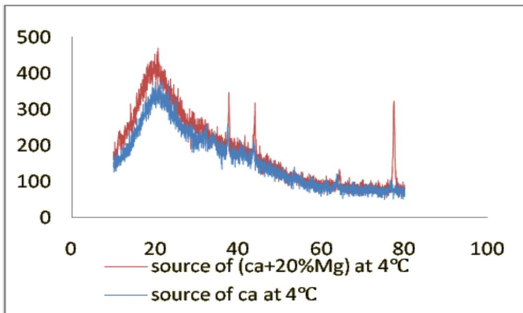
**Figure 3.** XRD spectra for source of Ca and (Ca+20%Mg)
