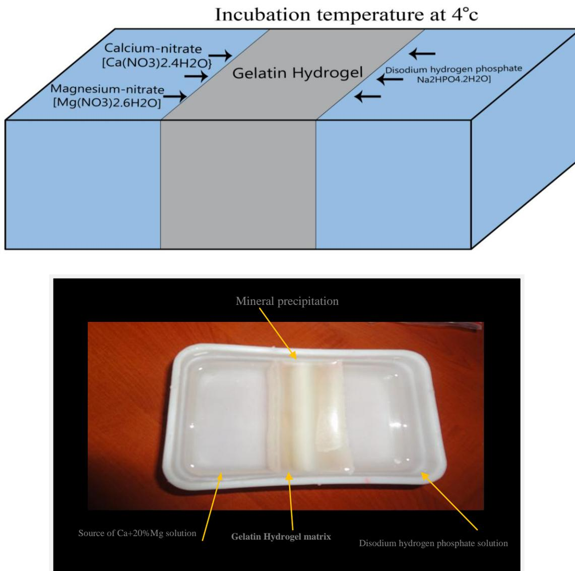
**Figure 1.** Schematic view of reactor used for bio mineralization of apatite within GEL hydrogel via double diffusion.
